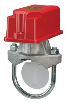
The new **WFDN Series** waterflow detectors from **Safe Signal** consists of a rugged, NEMA 4-rated enclosure that is more damage resistant than previous metal designs. The waterflow detector is designed for both indoor and outdoor use, with the widest available temperature range, from 32°F to 150°F. They are also approved for installation on the widest range of pipe schedules, sizes 2 in. through 4 in. are approved for installation on pipe schedules 7 through 40.
